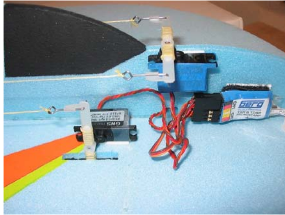
Servo setup showing string attachment to the control horns.
