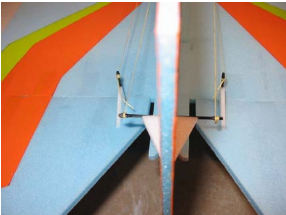
Kevlar string is just glued to the carbon rod.
