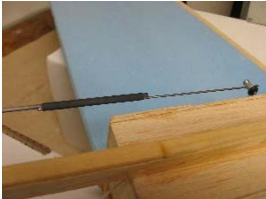
The wire is glued to the carbon rod, and heat shrink is over the wire. A drop of CA is placed at each end of the heat shrink.
