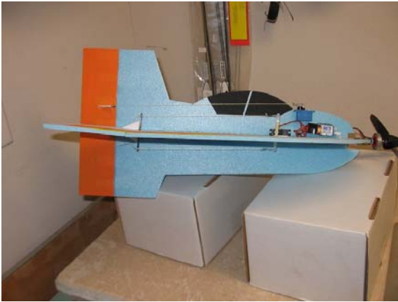
Complete pull/pull setup. The servo arm is above and below the wing, allowing pull for up and down.
