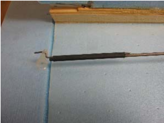
Wire attached to the carbon rod. A Z-bend is used to attach to the control surface.
