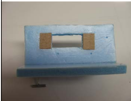
1/64 ply (or stiff balsa) glued into place
