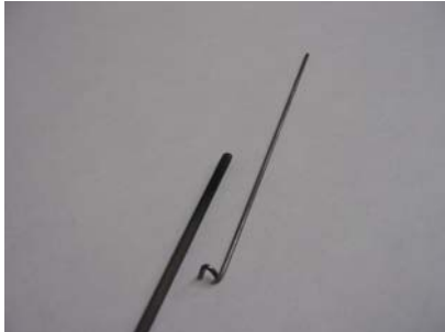
1) Bend a small right angle loop into the axle wire, which will hook onto the carbon fiber landing gear.
