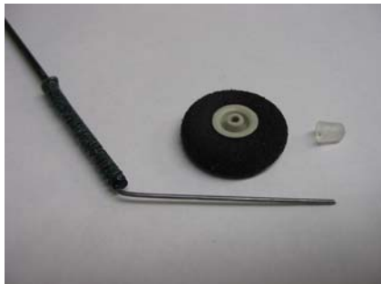
3) Landing gear ready for assembly. Bend wire 45 degrees to form axle for wheel.
