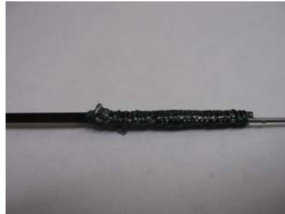
2) CA the wire to the carbon rod, then secure in place by wrapping with Kevlar string, then apply CA to the string wrap.
