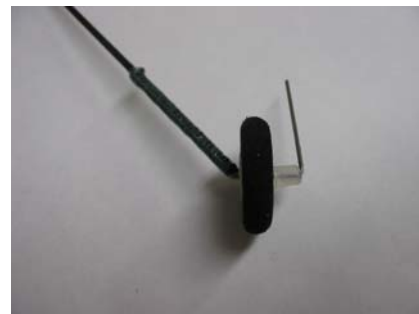
4) Slide on wheel, add small plastic spacer, then bend wire to hold wheel in place.
