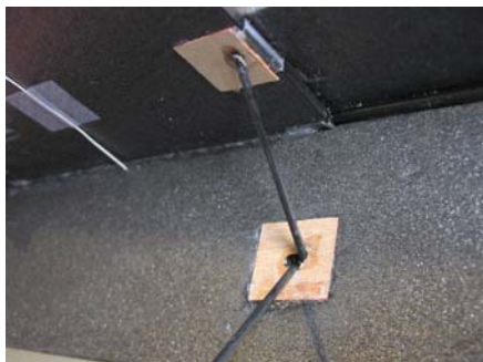
5) Landing gear passes through fuse, and is supported with thin ply that has been glued in place.
