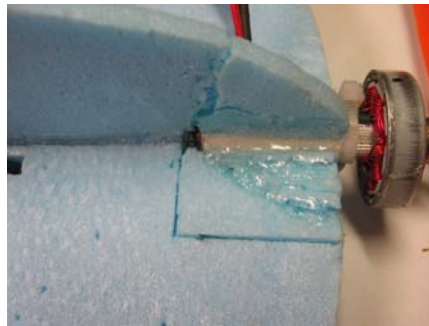
Photo #2 (cut out damaged area)
