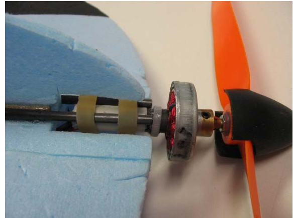
Bottom view Latex bands loop over motor and carbon tubes
