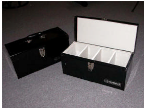
Charge box for Li Po batteries.
