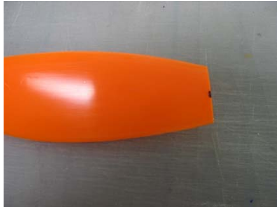
Cut, but not sanded. Just snap along the Knife score mark.
