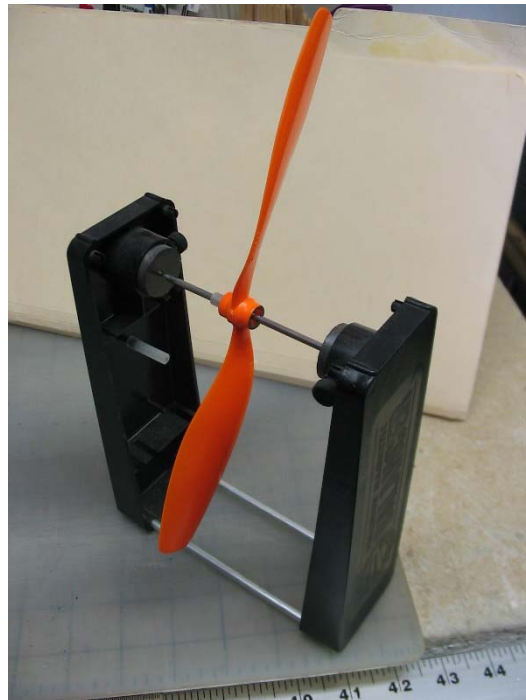
Balance prop after any modifications.
