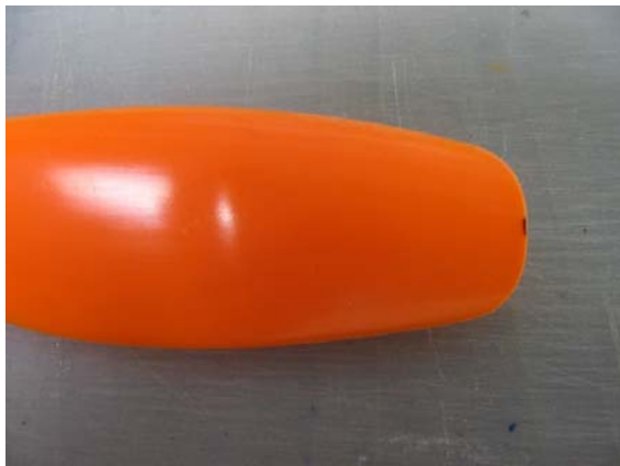
Sand to desired shape.
