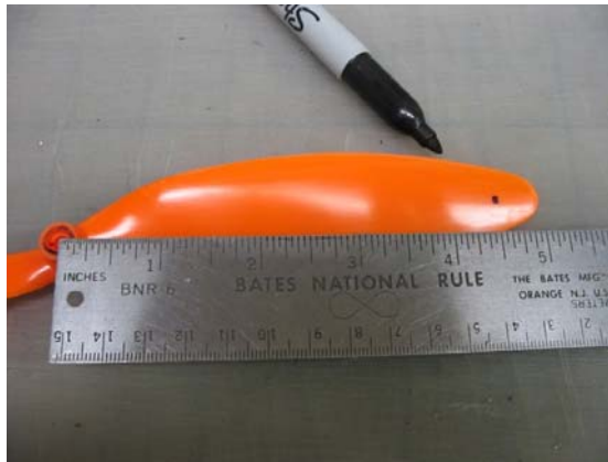
Measure 4.5" from the hub, and mark.
