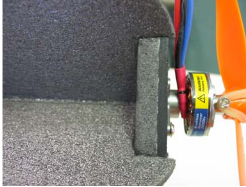
The foam is glued directly to the plane. In this particular installation, the nose was recessed to accept the foam/ply mount.
