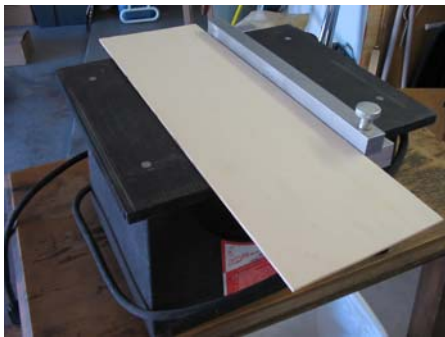
Using a stable small table, I cut 1/8" light ply into 1.5" x 1.5" sq.
