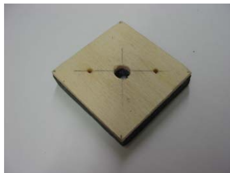
The mount is marked and drilled for the motor.
